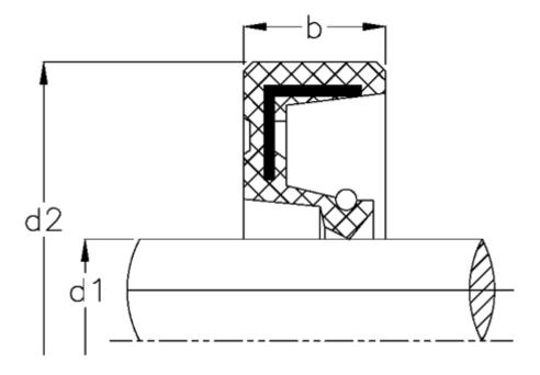
$\begin{array}{ll} b & = 12 \\ d1 & = 65 \\ d2 & = 85 \\ Material = NBR \end{array}$
